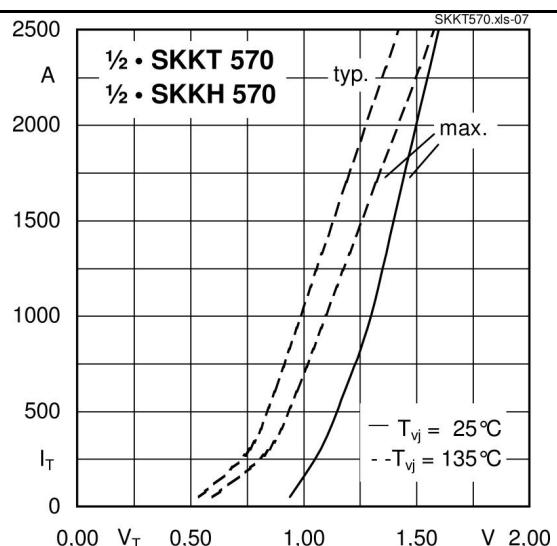
Fig. 7 On-state characteristics
